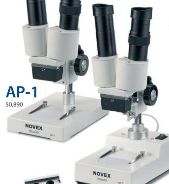
The AP-1 and AP-2 stereo microscopes have a vertical binocular head with dioptre adjustment and adjustable eye separation of 55 to 75 mm. Focussing movement is adjusted by two knobs via a transmission clutch. The stand is made of light metal and is supplied with black-white stage plate.
